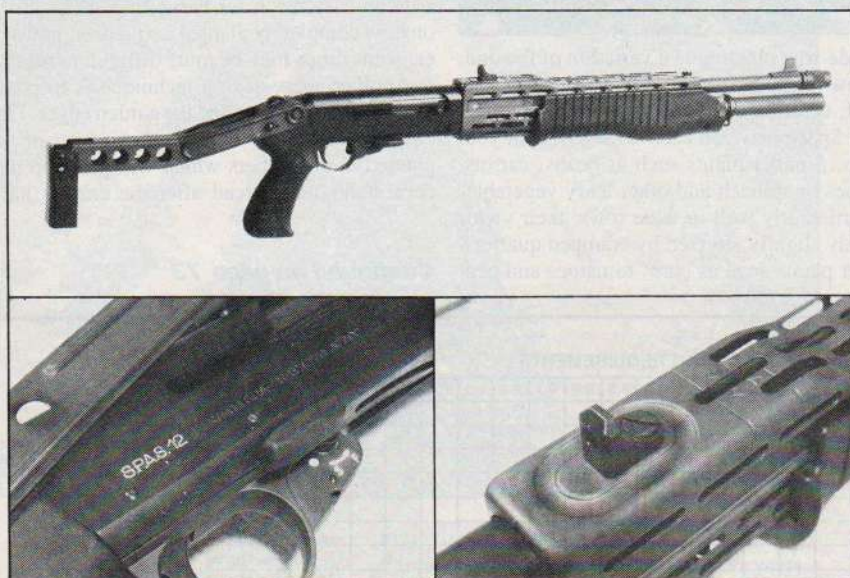
ABOVE LEFT: Carrying safety blocks the trigger; rotates 180 degrees to the fire position. ABOVE RIGHT: Aperture rear sight also retains the folding stock. Letters AA and MM serve as an operating-mode reference by their relation to the rear of the handguard.
