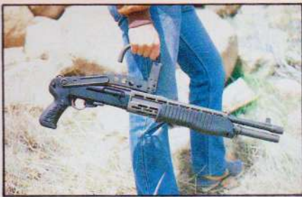
SPAS-12 with buttstock folded and locked against top of receiver. One-hand firing brace can also serve as a carrying handle.
