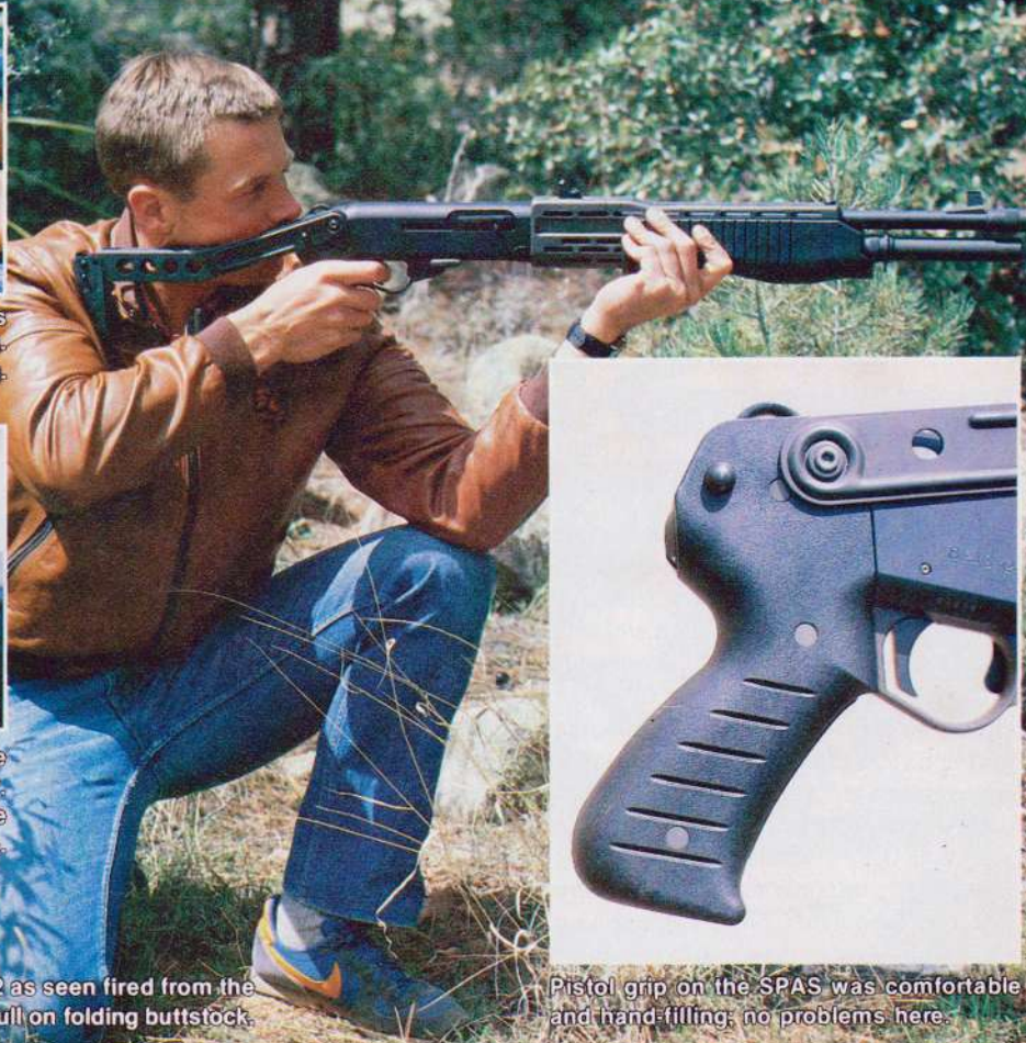
Adjustable semi-circular metal brace is designed for one-handed firing. Awkwardness of manual safeties, however, precluded using gun in this fashion.
