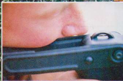
Stamped-metal buttstock caused extreme discomfort when fired from the shoulder. Attachment point for carrying sling can be seen immediately in front of shooter's nose.
