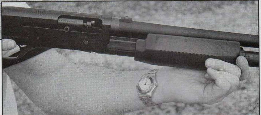
Firing mode for the Benelli M3 is switched by turning the selector ring.
