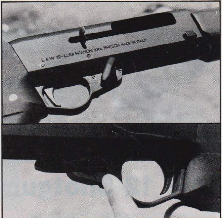
The main safety is the carry safety, a knob that points forward for "fire" and 180 degrees to the rear for the "on safe" position. On the opposite (right) side of the trigger guard is the quick employment safety which is moved forward for the "fire" position and back for "safe."
