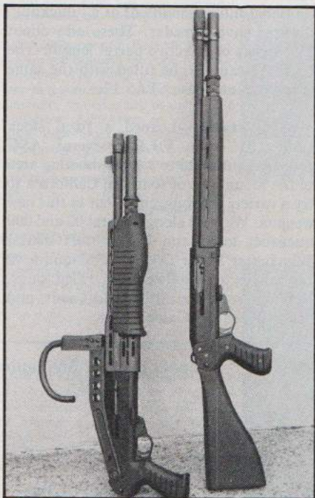
The LAW 12, right, is sold in fixed stock model only but can be converted after purchase to use a folding stock like that of its predecessor, the heavier, more complicated SPAS 12.
