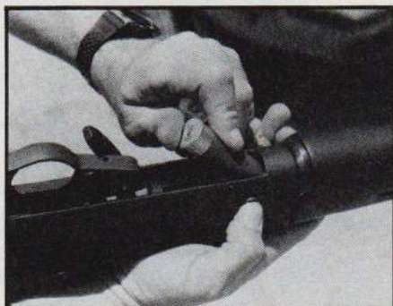
Loading is easiest with the gun cocked. Make sure safety is on and chamber is empty.
